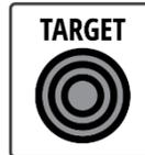
The TARGET PROGRAMS key launches the Target Program setup mode. The user can program a custom calorie, time or distance target.
