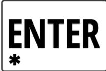
The ENTER key confirms a value to be entered when adjusting a program. Pressed in conjunction with the ENTER key, the Setup Mode will launch. To launch the Comp Mode, press the ENTER key for five seconds.
