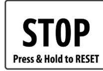
Use the STOP key to *end* a program or temporarily *pause* a running program. To reset the console and erase all user-entered data, press the STOP key for more than two seconds.
